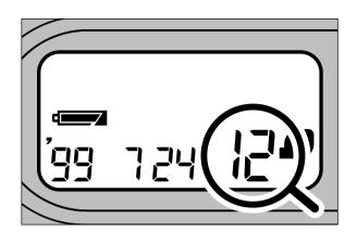
When a cartridge that was removed in mid-roll  $\bigcirc$  is re-loaded, the film will automatically be advanced to the first unexposed frame. After that, operation is as before.
